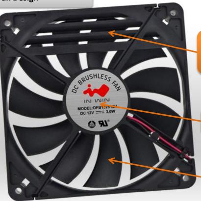
Proper fins to direct the air into the PSU! NOT a cheap plastic cover.
