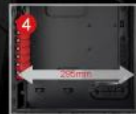
Sufficient depth of chassis for installing long cards
