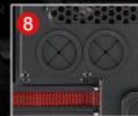
Pre-drill pipe holes for water cooling
