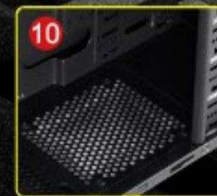
Can install 1x12 cm fan at bottom of case
