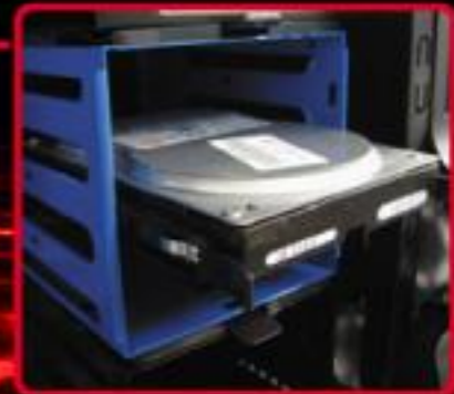
HDD cage fits three HDDs (screwless)
