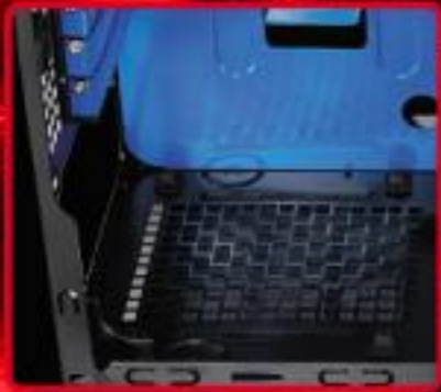
Filter included to prevent dust from entering PSU
