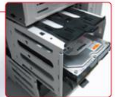
HDD cage fits three HDDs (screwless)
