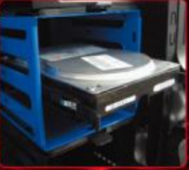
HDD cage fits three HDDs (screwless)
